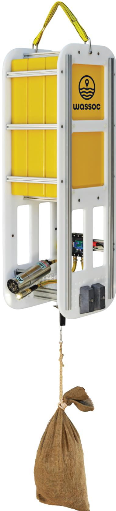
The Solo X Autonomous Benthic Lander (ABL) is a compact, water column and seabed observation platform. During deployment, the integral Solo X Subsea Imaging System captures video or imagery, logs data and ultimately releases the sacrificial anchor returning the ABL to the surface.
